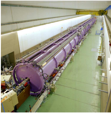
(a) Photo of the UNILAC accelerating structure [100].
