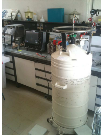
Figure 2.26: Photo of the experimental setup of the diamond test in LHe. The white Dewar filled with LHe is in the foreground.
