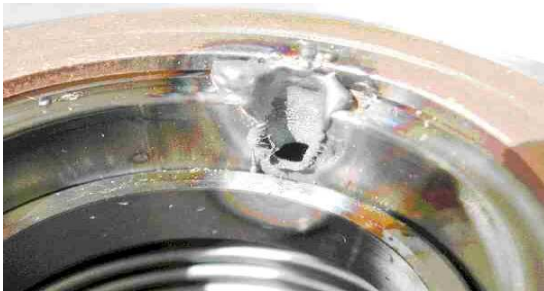
(a) Damaged inflicted to the beam pipe by the high-power electron beam of the ELBE accelerator [45].
