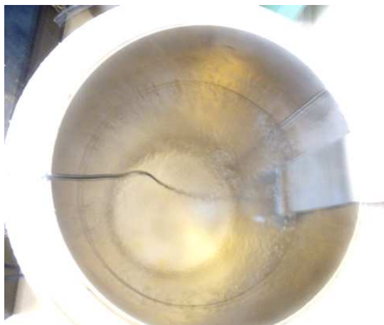
Figure 2.24: Photo of the CVD diamond test in liquid nitrogen with a ^{252}\text{Cf} source outside the Dewar.
